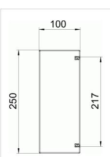
Sheet steel duct with intumescent interior coating In case of fire, actively prevents the spread of fire in the duct and protects emergency and escape routes against the impacts of a cable fire. The cover and base are securely interconnected using the self-contacting patented locking brackets. This also creates the equipotential bonding.
