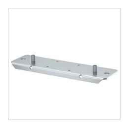
Support profile for suspended mounting of BSKM 0711, suitable as a suspension point to accept two M10 threaded rods and as the counterbearing to seal the joint, including nuts.
