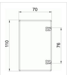
Sheet steel duct with intumescent interior coating In case of fire, actively prevents the spread of fire in the duct and protects emergency and escape routes against the impacts of a cable fire. The cover and base are securely interconnected using the self-contacting patented locking brackets. This also creates the equipotential bonding.
