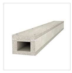
Fire protection duct for fire-proof routing of photovoltaic cables and inside and outside buildings. Consists of non-conductive, frostresistant fibre glass lightweight concrete and fulfils the requirements for the contact protection of rescue services in case of fire. Tested and approved to DIN 4102 Part 11, as an I30 duct, may therefore be used in emergency and escape routes. Including lid screws and 3 m of sealing strip.
